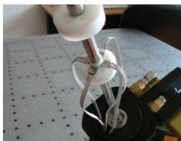
Fig. 14. Teflon rings used to mount the microphones flush with the tube wall.
